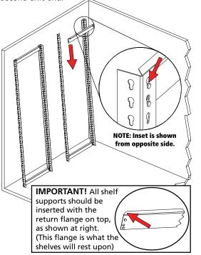
2. Next, connect the two unit ends with two LRA left-to-right shelf supports (Ref. No. 3), temporarily leaving off one of the top left-to-right supports.
