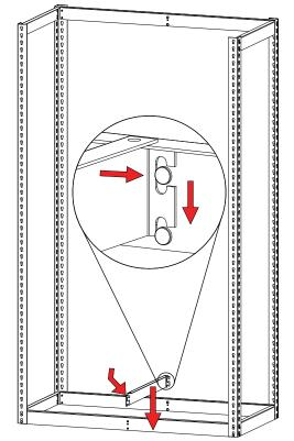
**4.** Lay the bottom shelf decking (Ref. No. 5) on the shelf supports so that the front and back edges overlap the front and back shelf supports.
