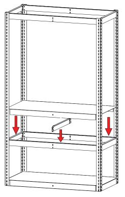
NOTE: Every fourth slot in the uprights has a flat top to help visually align the supports.
