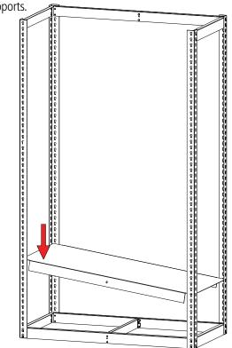
**5.** Attach shelf supports at the next desired shelf level. Once the shelf supports are in place, attach a front-to-back center supports as you did in step 3. Lower the steel decking into place, as described in step 4.
